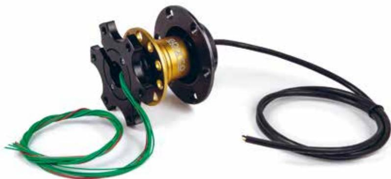
/ Wire harness with silver solder connection with LEMO connectors from F1.
